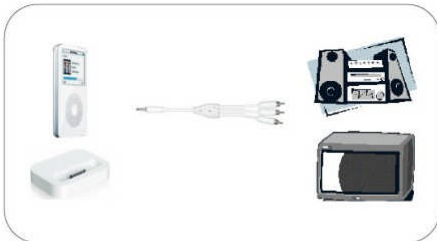
Illustration of the iPod and A/V Cable connection. Note: Video (Yellow) and Audio (Red and White) colors .
